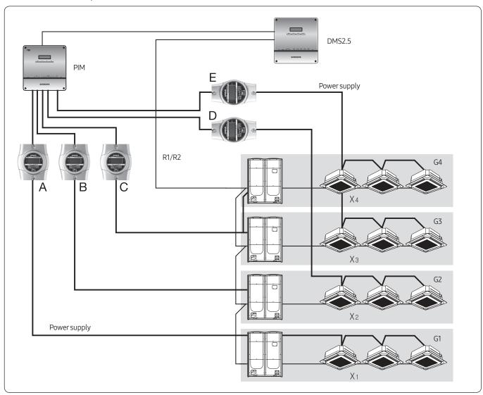
• When configuring the DMS2.5 and the whole system, mapping of watt-hour meters for indoor/outdoor units must be precisely assigned for correct power distribution.
