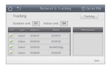
• Indoor unit with no check mark on S/H (Show/Hide) check box, will not be controlled and monitored from the Touch centralized controller.
