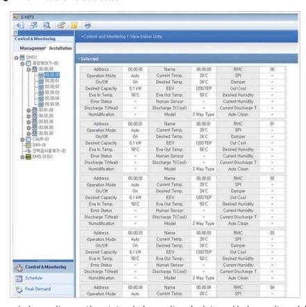
• Indoor unit operation status, indoor unit cycle data and indoor unit model code is displayed.
