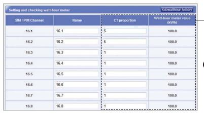
[Setting and checking watt-hour meter] From the menu, CT proportion of the CT watt-hour meter must be entered.
