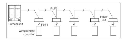
Only when the wired remote controller is connected to an indoor unit directly (1:1 connection), you can set the mode master indoor unit that sets the operation mode of the outdoor unit.
