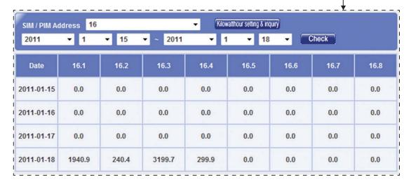
• Setting virtual watt-hour meter When watt-hour meter or PIM interface module is not installed to a watt-hour meter channel, virtual channel can be used to manually distribute the power distribution
