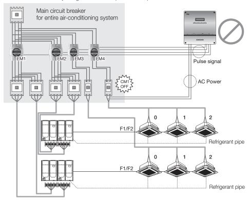
• Example 2) Even when the circuit breaker, CM1 is switched off while the others are on, pulses from the electricity meters, EM1, EM2 and EM3 are still calculated by MIM-B16N, whose power is not interrupted by CM1.
