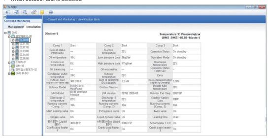
· Outdoor unit cycle data, outdoor unit model, interface module model and interface module program version is displayed.
