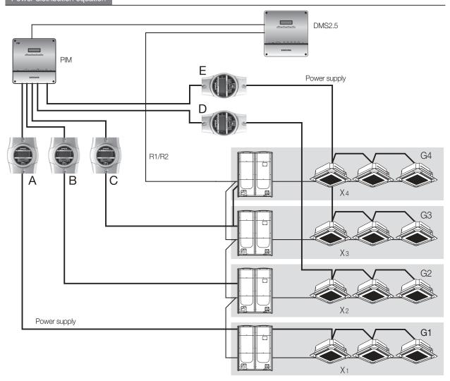
▶ When configuring the DMS2.5 and the whole system, mapping of watt-hour meters for indoor/outdoor units must be precisely assigned for correct power distribution.
