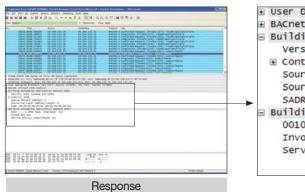
■ User Datagram Protocol, Src Port: bacnet (47808), BACnet Virtual Link Control Building Automation and Control Network NPDU Version: 0x01 (ASHRAE 135-1995) ⊕ Control: 0x08 Source Network Address: 1 Source MAC Layer Address Length: 6 SADR: 80:00:00:0b:00:01 (80:00:00:0b:00:01) Building Automation and Control Network APDU 0010 .... = APDU Type: SimpleACK (2) Invoke ID: 121 Service Choice: subscribeCOV (5)
