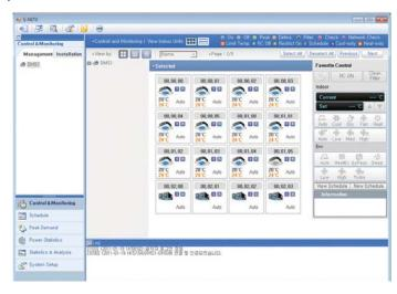
PC program designed to manage system air conditioners in a large site.
