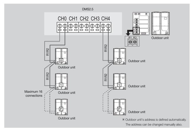
Connecting with OnOff controller / Touch centralized controller
