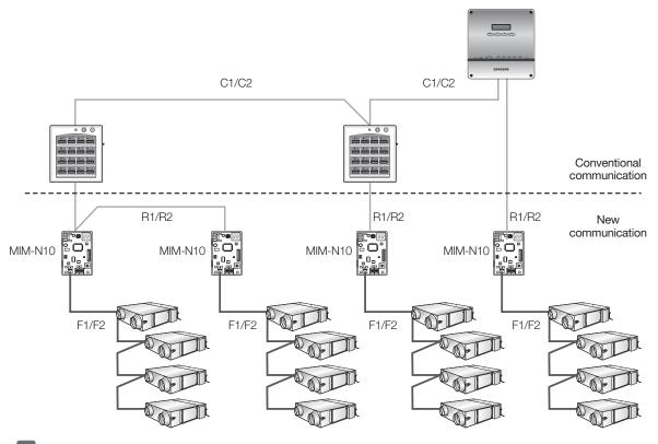
Conventional/new communication ERV ↔ New communication upper level controller
