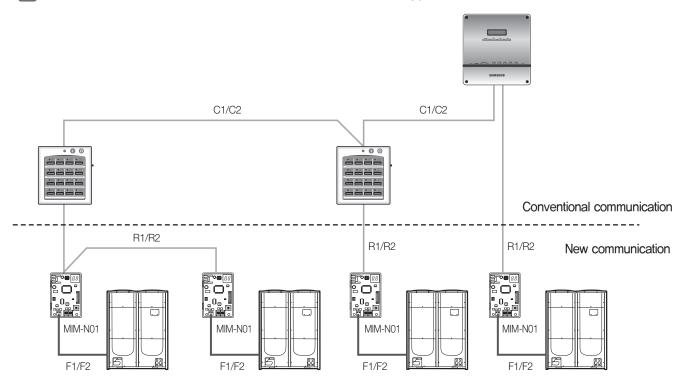
Conventional communication outdoor unit ↔ New communication upper level controller
