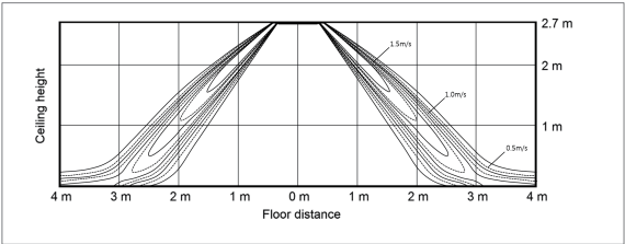
Cooling Air Velocity distribution
