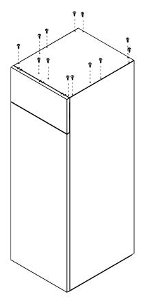
1 Remove 13 mounting screws from the Top Plate.
