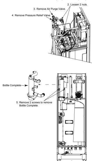
18.9 To Remove Anode Bar
