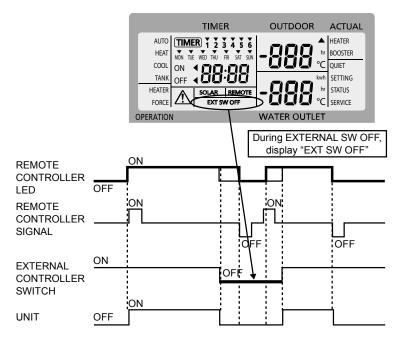
\* During External Switch OFF condition, it is allow to change the setting and also timer operation.
