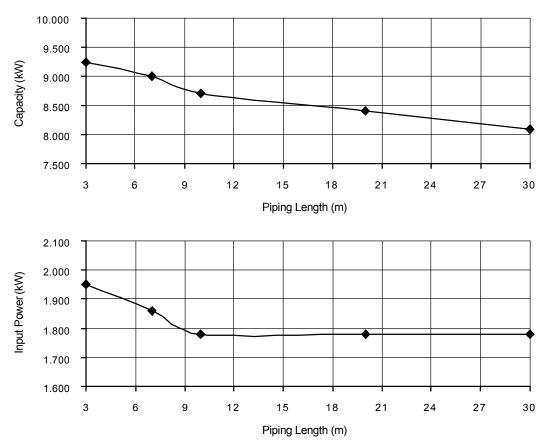
Cooling Characteristics at Different Piping Length Condition Outdoor air temperature : 35°C (DBT), -°C (WBT) Indoor water inlet temperature : 12°C Indoor water outlet temperature : 7°C Piping length : 7 m
