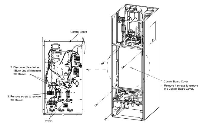
18.5 To Remove Transformer and Electronic Controller
