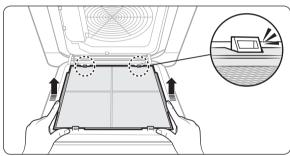
Pull out the air filter from the indoor unit.
