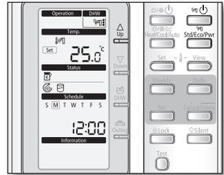
2. Press **Mode (DHW mode)** button until required operating mode is displayed.
