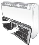
4. Clean the Air filter with a vacuum cleaner or soft brush. If dust is too heavy, then rinse it with running water and dry it in a ventilated area.
