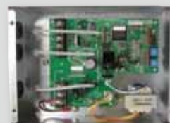
BMS-IFWH5E For Energy Monitoring
