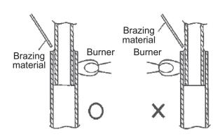
The pre-heating is to heat the base material until the melting temperature, and requires certain training to distinguish the color of the heated base material in order not to melt the material.
