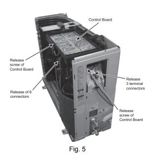
7. Remove the 4 screws of the Electronic Controller.
