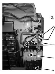
2. Release the 2 screws of the earth grounding terminal.
