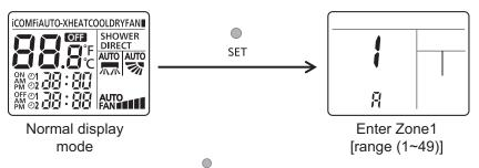
4 To enter zone 2 area: (Press set continuously for T ≥ 5 secs)
