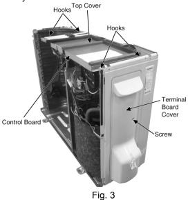
5 Remove the Control Board as follows:
