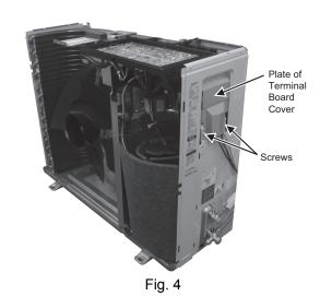
6 Remove the Control Board.
