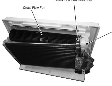
3. Release the 4 screws of the Fan Motor. Fan Motor can be removed after the removal of the Cross Flow Fan
