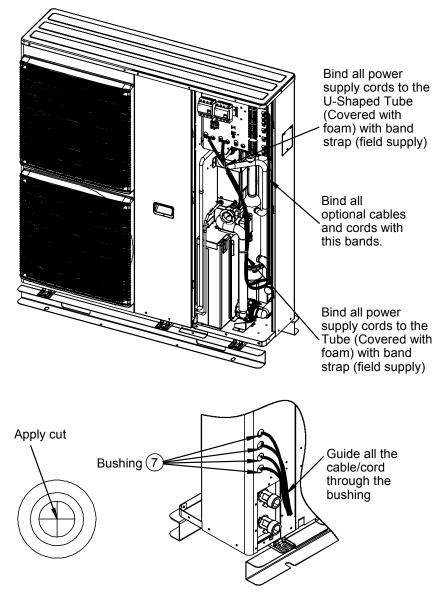
How to guide cable/cord to bushing
