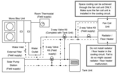
Diagram 3.1: Typical Water Piping Installation
