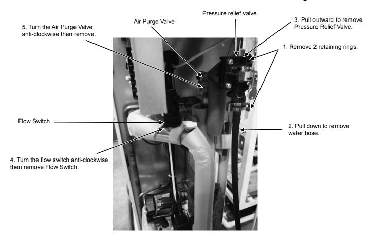
⚠ When reinstall Flow Switch, ensure the arrow on the flow switch is parallel with the pipe shaft and is facing in the direction of flow.
