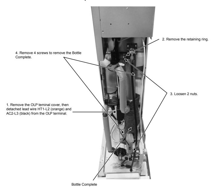
⚠ When reinstall the water pipe, use grease or water at the joining.
