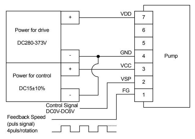
Control signal is analog voltage (DC0V-6V) generated by microcomputer PWM port. Microcomputer can change analog voltage by changing PWM duty.
