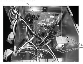
② Remove 4 screws to remove Transformer.
