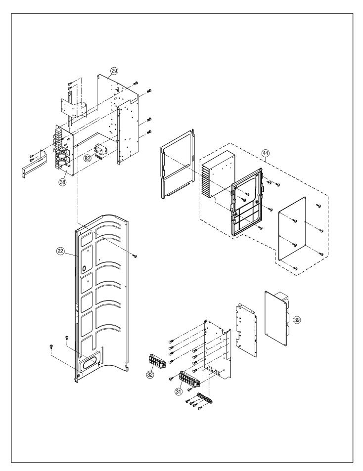
The above exploded view is for the purpose of parts disassembly and replacement. The non-numbered parts are not kept as standard service parts.
