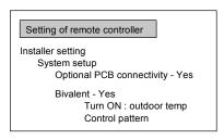
This is an application that connects the boiler to the indoor unit, to compensate for insufficient capacity by operate boiler when outdoor temperature drops & heat pump capacity is insufficient.
