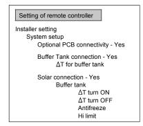
This is an application that connects the buffer tank to the indoor unit before connecting to the solar water heater to heat up the tank.
