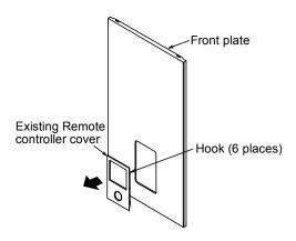
2. Press from front to fix the Remote controller cover 6 on the front plate.
