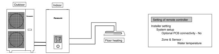
Connect floor heating or radiator directly to the indoor unit.
