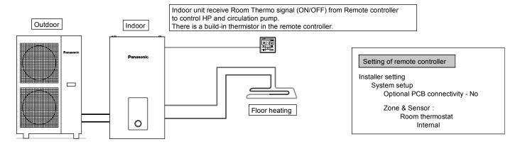
Connect floor heating or radiator directly to the indoor unit.
