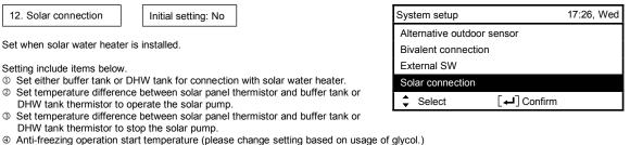
Solar pump stop operation when it exceeds high limit temperature (when tank temperature exceed designated temperature (70~90°C))
