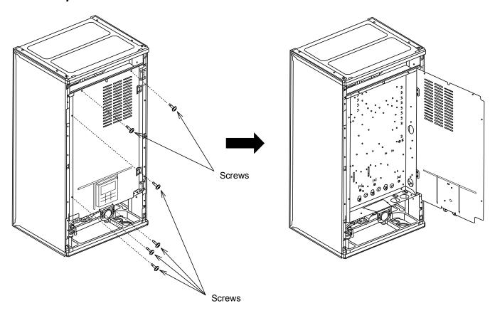
1. Remove 6 screws from the Control Board Cover.
