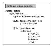
This is an application that connects the buffer tank to the indoor unit before connecting to the solar water heater to heat up the tank.
