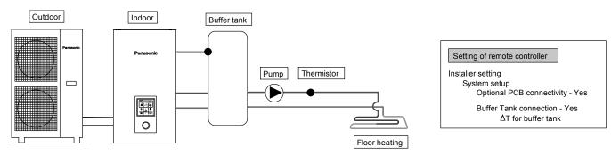
This is an application that connects the buffer tank to the indoor unit.
