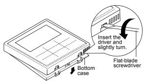
Remove the wiring between Remote controller and Indoor Unit terminal. Remove the bottom case from the Control board cover by loosening the screws. (3 pieces)
