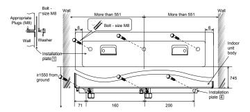
The centre of installation plate should be at more than 551 mm at right and left of the wall.
