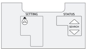
These 3 SW's should press continuously for 5secs. (Operation should be OFF during this period)
