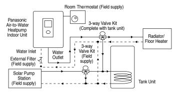
Diagram 4.1: Typical Water Piping Installation
