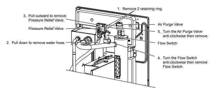
When reinstall Flow Switch, ensure the arrow on the flow switch is parallel with the pipe shaft and is facing in the direction of flow.
