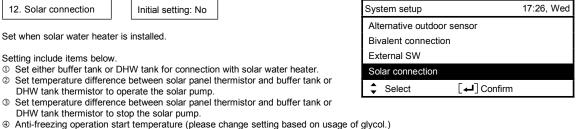
Solar pump stop operation when it exceeds high limit temperature (when tank temperature exceed designated temperature (70~90°C))
