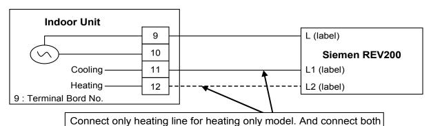
heating and cooling line for heat + cool model.
