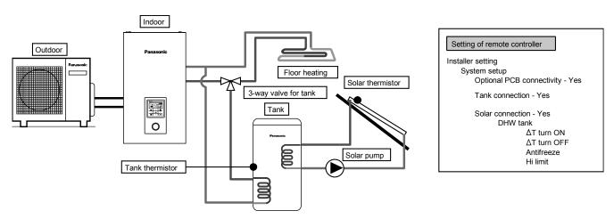
This is an application that connects the DHW tank to the indoor unit through 3-way valve before connect the solar water heater to heat up the tank. DHW tank's temperature is detected by tank thermistor (specified by Panasonic). Solar panel's temperature is detected by solar thermistor (specified by Panasonic).
