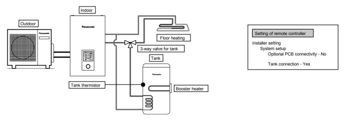
This is an application that connects the DHW tank to the indoor unit through 3-way valve. DHW tank's temperature is detected by tank thermistor (specified by Panasonic).
