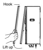
Fix the left and right hooks to cabinet slot properly when reinstall front plate.
