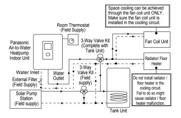
Diagram 4.1: Typical Water Piping Installation
