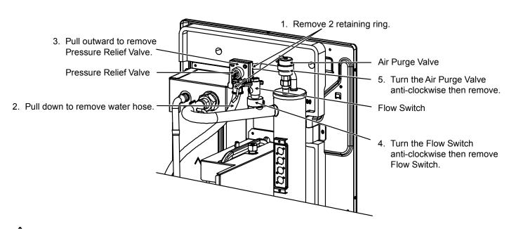
When reinstall Flow Switch, ensure the arrow on the flow switch is parallel with the pipe shaft and is facing in the direction of flow.
