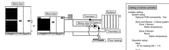
This is an example of simple 2 zone control without using buffer tank.
