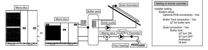
This is an application that connects the buffer tank to the Mono bloc before connecting to the solar water heater to heat up the tank.
