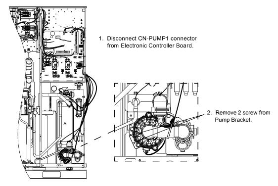
Mhen reinstall the water pipe, use grease or water at the joining.
