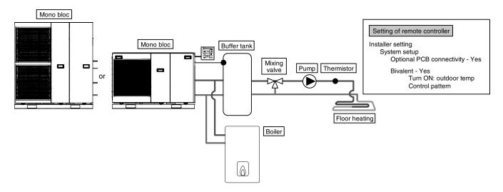
This is an application that connects the boiler to the Mono bloc, to compensate for insufficient capacity by operate boiler when outdoor temperature drops & heat pump capacity is insufficient.
