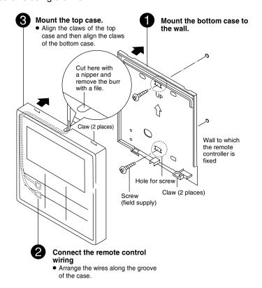
Preparation: Make 2 holes for screws using a driver.
