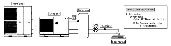
This is an application that connects the buffer tank to the Mono bloc. Buffer tank's temperature is detected by buffer tank thermistor (specified by Panasonic). This system requires optional PCB (CZ-NS4P).
