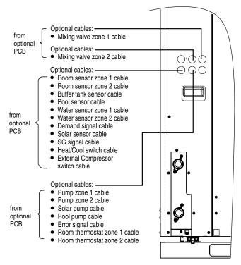
How to guide optional cables to bushing 15
