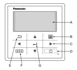
Name Function Main screen Display information A: B: Menu Open/Close main menu C: Triangle (Move) Select or change item D: Operate Start/Stop operation E: Back Back to previous item F: Quick Menu Open/Close Quick menu OK Confirm G:
