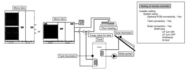
This is an application that connects the DHW tank to the Mono bloc through 3-way valve before connect the solar water heater to heat up the tank. DHW tank's temperature is detected by tank thermistor (specified by Panasonic). Solar panel's temperature is detected by solar thermistor (specified by Panasonic).
