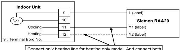
Connect only heating line for heating only model. And connect both heating and cooling line for heat + cool model.
