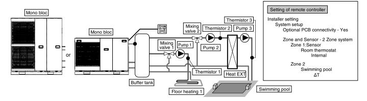
Connect floor heating and swimming pool to 2 circuits through buffer tank as shown in figure.
