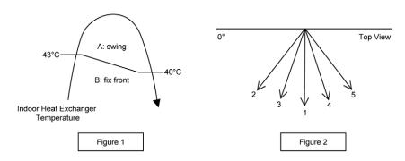
Manual horizontal airflow direction can be set using remote control; the angles of the vane are as stated below and the positions of the vane are as Figure 2 above.
