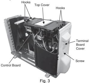
5 Remove the Control Board as follows:
