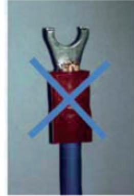
Terminal has been cut.
