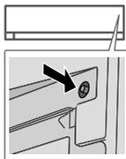
Use when remote control is misplaced or a malfunction occurs. Raise the front panel:
