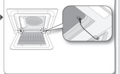
Clean the grille and Air filter with a vacuum cleaner or soft brush. If dust is too heavy, then rinse it with running water and dry it in a ventilated area.
