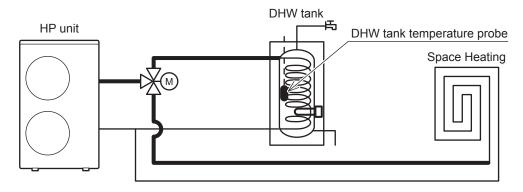
The DHW can be heated as following configuration by setting Par3102.
