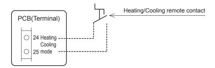
Note: Heating/Cooling remote contact will be used when the operation of HP unit is turned ON by ON/OFF remote contact. It is not available if ON/OFF remote contact is OFF, and set Par5120=0.
