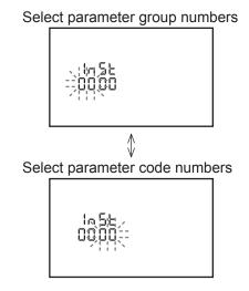
3 In INSTALLER level, more parameters than USER level can be accessed.
