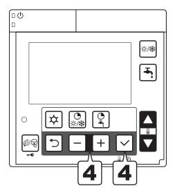
When the day of the week has been saved, the time band operation ON/OFF (Default: off) blinks. Specify either "on" or "off" using the - or + button and then press the Set button to save the setting.
