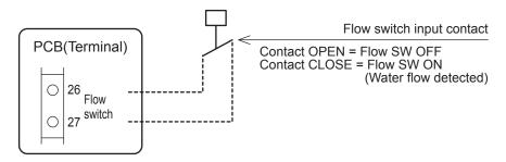
At Start-up, the compressor will not be turned ON unless the flow switch is CLOSED (water flow detected).
