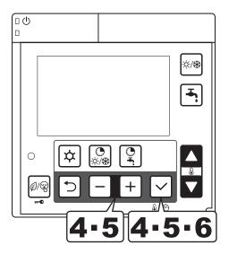
When DHW Comfort/Economy set point has been saved (in Low tariff or Night mode, when the mode selection has been saved), "1 On" displays and "0:00" blinks; set the 1st ON time. When the - or + button is pressed, the time changes in 15 minute increments. Press the Set button to save the setting.
