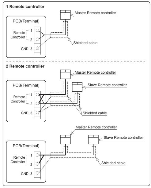
The maximum length of the Remote controller cord is 100m.
