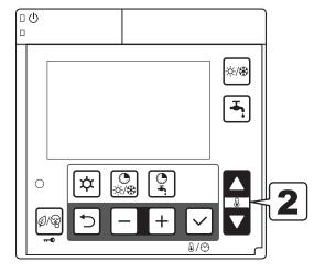
2 Press the Up or Down button to set the desired room set temperature.
