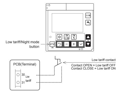
Note1: Par5128 (Night mode) and Par5130 (Low tariff) are automatically synchronized to same value. If Par5128 is changed to 1 (enable), then Par5130 will be also changed to 1 (enable).
