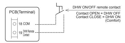
Note1: DHW function can be used by the DHW remote contact.
