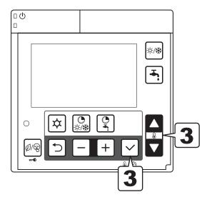
3 Select the group and code numbers by pressing the Up or Down button, and press Set button to display the parameter value in the display.
