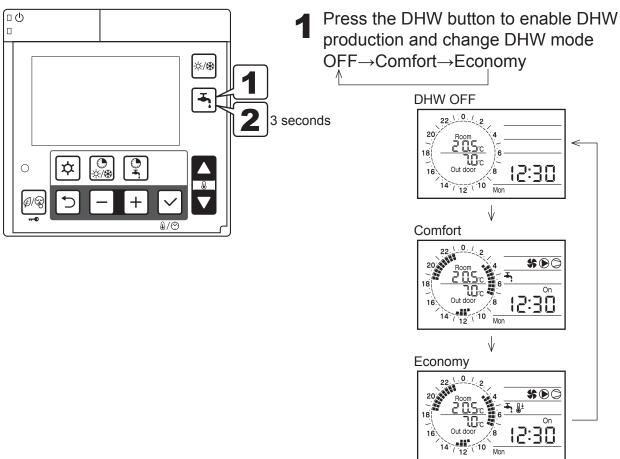
Press the DHW button for 3 seconds to enable DHW Force mode. In Force mode, hot water will be supplied to DHW tank until the DHW tank temperature reaches the Over boost set point. Force mode will be available until it is disabled by pressing the DHW button for 3 seconds.
