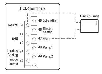
In case of Par0400=1, if the Room air temperature detected by the Remote controller has not reached the set point, the Terminal47 will be closed.
