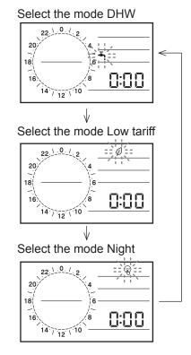
Note: Press the Return button to return to the previous item. Press the Timer for DHW button for 3 seconds again to return to normal operation, or simply do nothing for approximately 2 minutes.
