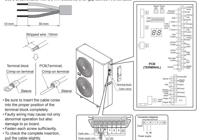
\*Swage the rod terminal of a lead to wire. Do not solder a lead, or it may cause a fire.
