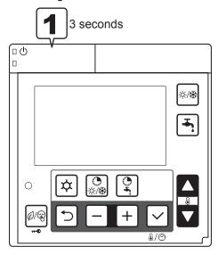
Press ON/OFF switch for 3 seconds to turn ON/OFF the system.
