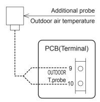
The maximum length of probe cables is 100m for 1mm<sup>2</sup> cables, and 30m for 0.5mm<sup>2</sup> cables.
