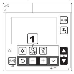
Push the Timer for Heating/Cooling button once to activate the time bands, once again to deactivate.
