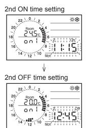
When the settings prior to the 3rd time band OFF time have been specified, the relevant day of the week setting is complete, and it returns to step 2. Then, set other zones and other day of the week.
