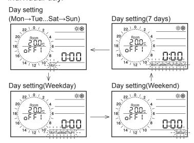
Note: Press the Return button to return to the previous item. Press the Timer for Heating/Cooling button for 3 seconds again to return to normal operation, or simply do nothing for approximately 2 minutes.
