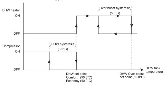
The DHW set point is reached (Comfort or Economy) using the compressor, the Over boost set point will be achieved with the DHW heater only and the HP unit will change over to the system.
