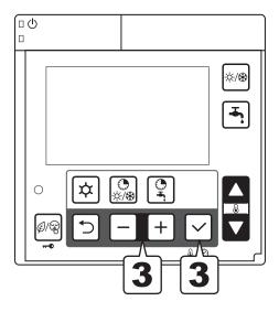
When the DHW Comfort icon displays and DHW Comfort set point (Default: 50°C) blinks, change the DHW Comfort set point using the - or + button, and press Set button to save the setting.
