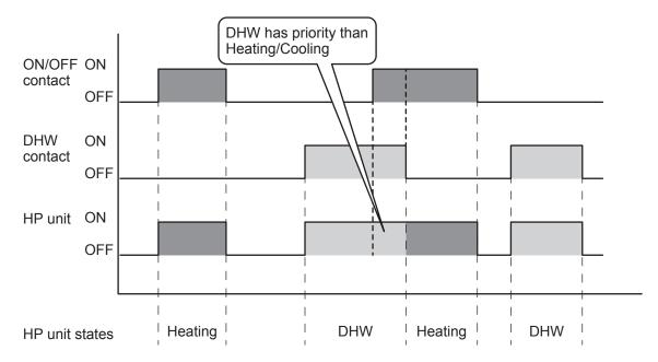
Note2: In case the ON/OFF remote contact is enabled and Heating/Cooling remote contact is disabled (by Remote controller), if the ON/OFF remote contact=ON and Heating or Cooling is in operation, and if the Mode button of Remote controller is used to select OFF among Heating→Cooling→OFF, the ON/OFF remote contact=ON condition will be top priority than the Mode button of Remote controller.
