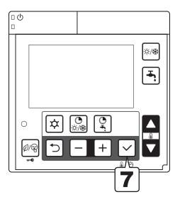
When the 1st ON time has been saved, "1 On" changes to "1 Off". Set the 1st time band OFF time. After entering the "OFF time", the gauge of the circle graph for ON time will be lighted, and then press the Set button to save the setting.
