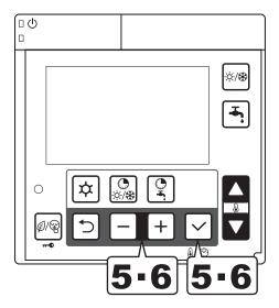
When the time band operation On/Off has been saved, Room set point for Heating/Cooling (Default: 20.0°C) blinks, Change the Comfort set point temperature using the - or + button, and press the Set button to save the setting.
