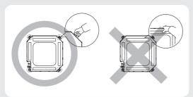
♦ Do not hold the discharge while carrying the indoor unit to avoid the possibility of breakage. You must hold the hanger plate on the corner and carry the indoor unit.
