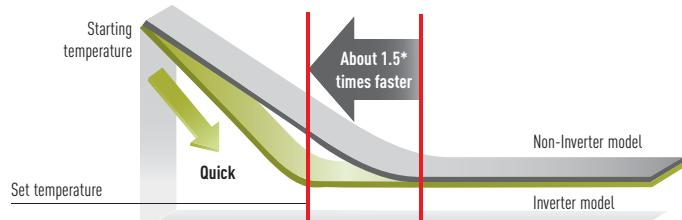
\* 1.5HP Inverter vs. non-Inverter. Outside room temperature: 35°C; setting temperature: 25°C
