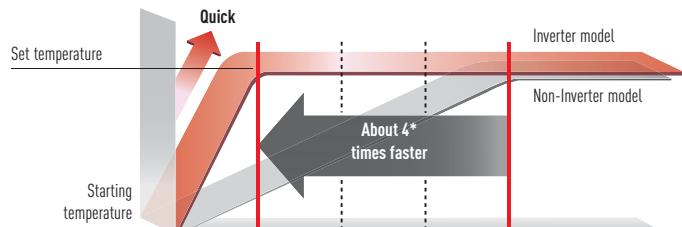
\* Comparison of 1.0HP Inverter and Non-Inverter. Outside room temperature: 2°C ; Setting temperature: 25°C
