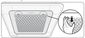
Push down the hooks at each side of the front grille to open the grille.
