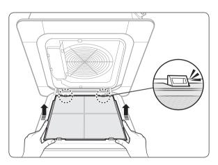
Pull out the air filter from the indoor unit.
