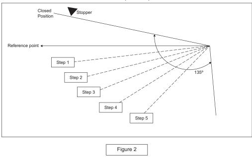
\* The horizontal vane angle tolerance is within +/- 5 degree.
