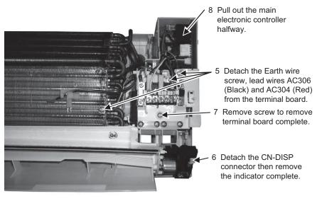
9 Detach connectors as labeled from the electronic controller. Then pull out main controller gently.
