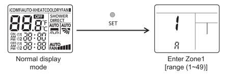
4 To enter zone 2 area: (Press set continuously for T ≥ 5 secs)
