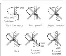
2 Pour water into the drain pan. Check whether the hose is well drained
