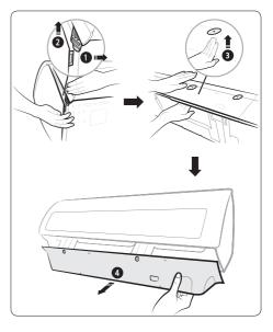
Step 2.2 Disassembling the installation plate
