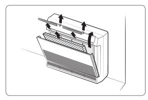
4 The body front should be opened to connect pipes.Please release the 4 screws of body front and then pull it out from the bottom of the set.
