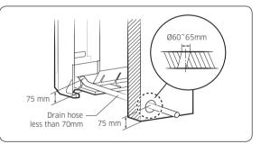
**6** The pipes & cable should be gone through the bottom back hole.
