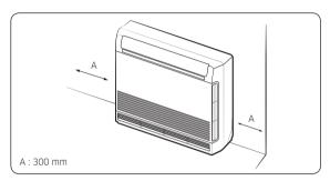
**2** When you install the indoor with side-pipe connection, please make space more than 300mm from the wall.
