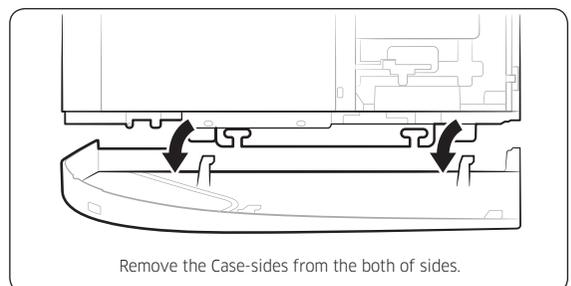
Remove the Case-sides from the both of sides.
