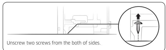
Unscrew two screws from the both of sides.
