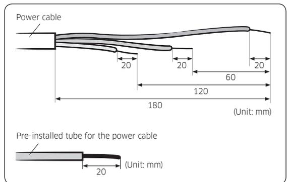
3 Insert both sides of core wire of the power cable into the connection sleeve.
