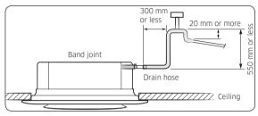
Do not give the hose an upward gradient beyond the connection port. This will cause water to flow backwards when the unit is stopped, resulting in water leaks.
