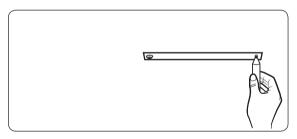
**3** Rotate the paper compass on its pivot point to draw a line on the ceiling.
