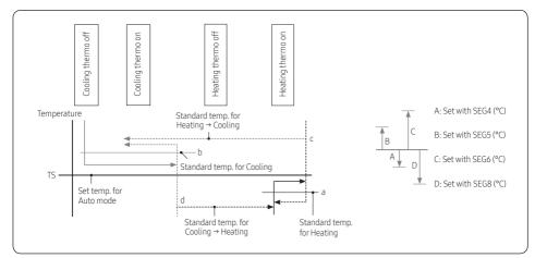
Cooling/Heating mode can be changed when Thermo Off status is maintained during the time with SEG9.
