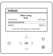
After cleaning and reassembling the air filter, be sure to reset the filter-cleaning reminder as follows :
