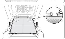
Pull out the air filter from the indoor unit.
