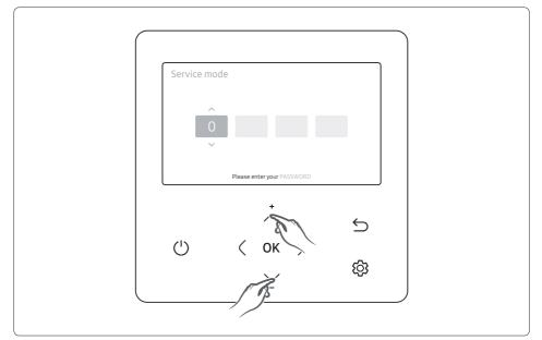
To set the indoor unit option code use the wired remote control and follow the directions below.
