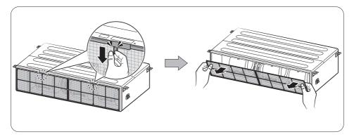
2 Clean the Air filter with a vacuum cleaner or soft brush. If dust is too heavy, then rinse it with running water and dry it in a ventilated area.
