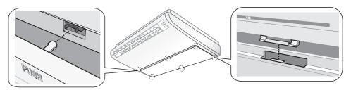
**3** Pull out the Air filter. Slightly press the air filter and then pull the air filter out.
