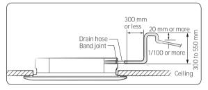
• Do not give the hose an upward gradient beyond the connection port. This will cause water to flow backwards when the unit is stopped, resulting in water leaks.
