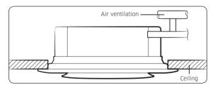
• If it is necessary to increase the height of the drain pipe, install the drain pipe straight within 300 mm from the drain hose port. If it is raised higher than 550 mm, there may be water leaks.
