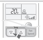
3 To adjust the temperature, press the  $\bigcirc$  buttons to set the desired temperature.
