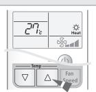
2 To select the Heat mode, press the Mode button until Heat is displayed on the remote control.
