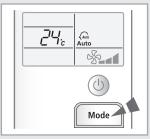
2 To select the Auto mode, press the Mode button until Auto is displayed on the remote control.
