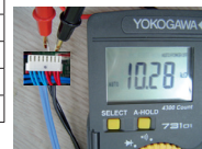
(Example) OLP sensor/discharge temperature sensor measuring resistance value by temperature: E320, E251.
