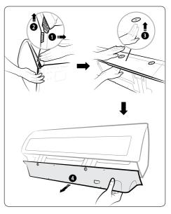
Step 2.2 Disassembling the installation plate
