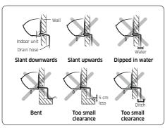
2 Pour water into the drain pan. Check whether the hose is well drained.
