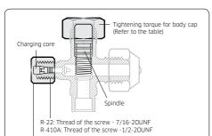
Tightening torque for charging port cap (Refer to the table)
