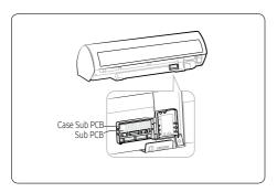
4 Find the PCB wire, and connect the wire to the Sub PCB as seen in the picture.
