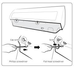
2 Unlock the side hooks (♠, ♠), then centre hooks (♠). Then unlock the bottom hooks (♠) to pull out the cover panel.
