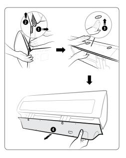
Step 2.2 Disassembling the installation plate
