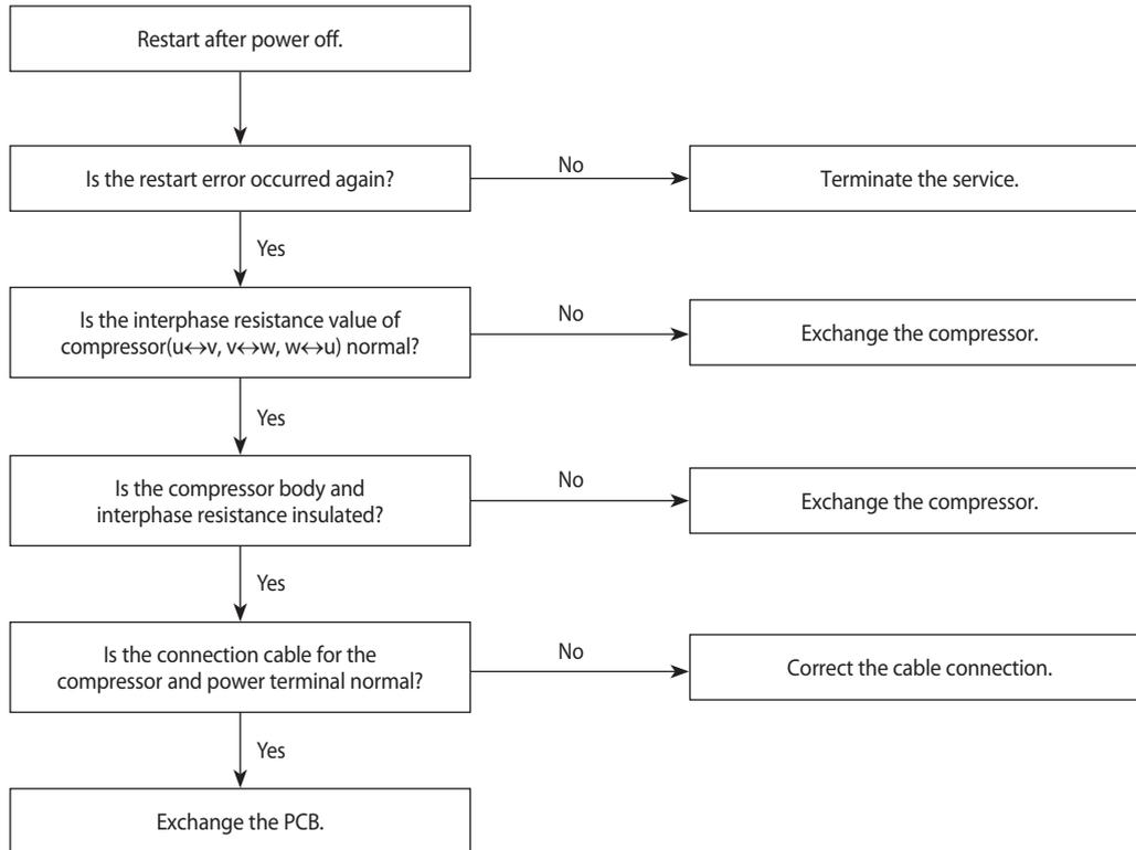
**4-4-18 E462 : Current protection control causes comp. down
