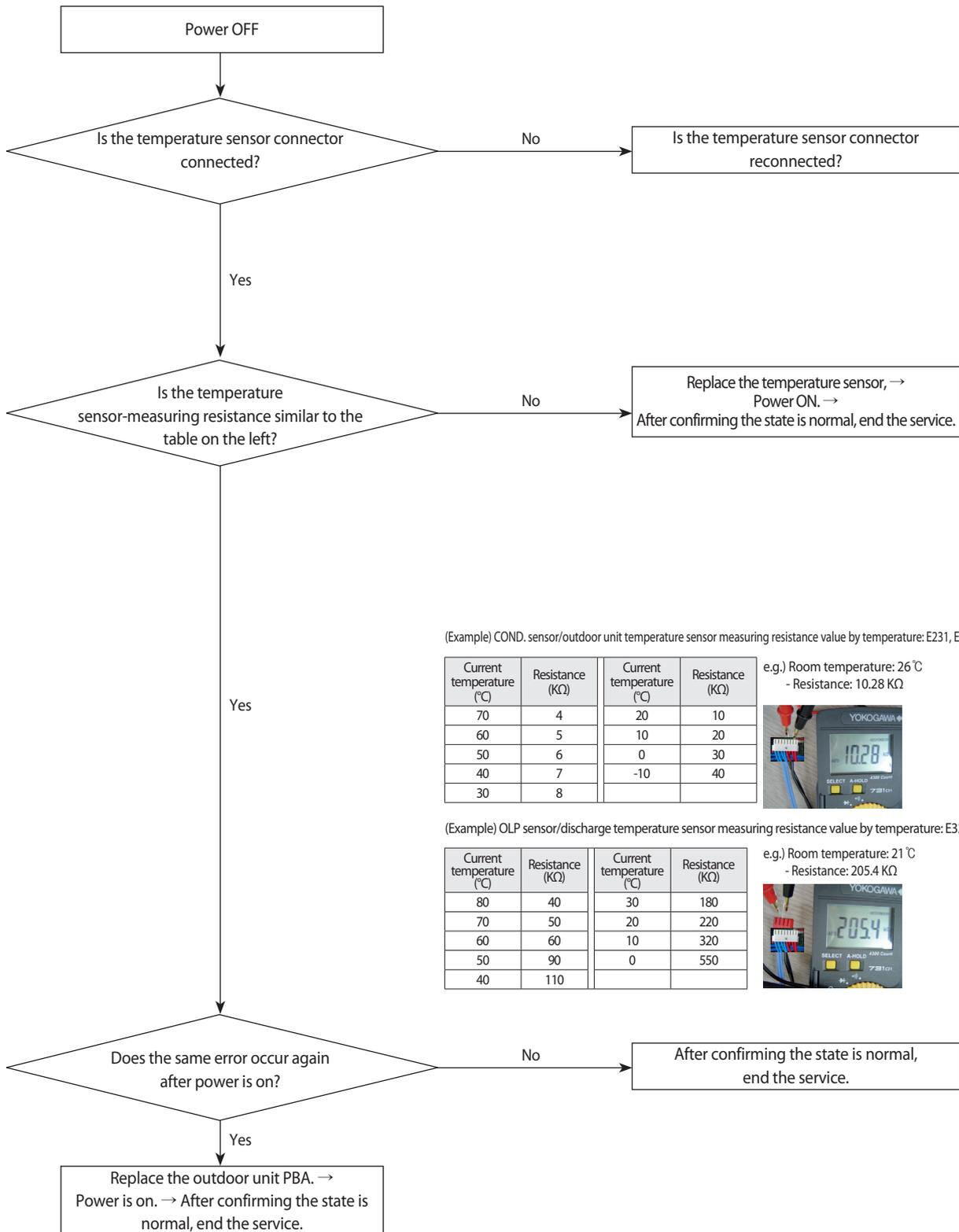
(Example) COND. sensor/outdoor unit temperature sensor measuring resistance value by temperature: E231, E221
