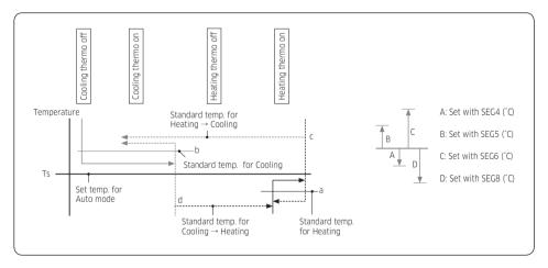
Cooling/Heating mode can be changed when Thermo Off status is maintained during the time with SEG9.
