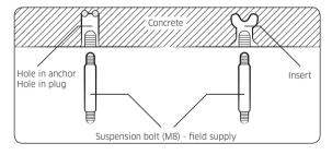
**3** Install the suspension bolts depending on the ceiling type.
