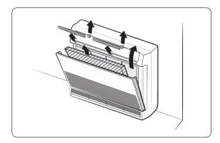
**4** The body front should be opened to connect pipes. Please release the 4 screws of body front and then pull it out from the bottom of the set.
