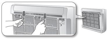
3. Clean the Air filter with a vacuum cleaner or soft brush. If dust is too heavy, then rinse it with running water and dry it in a ventilated area.
