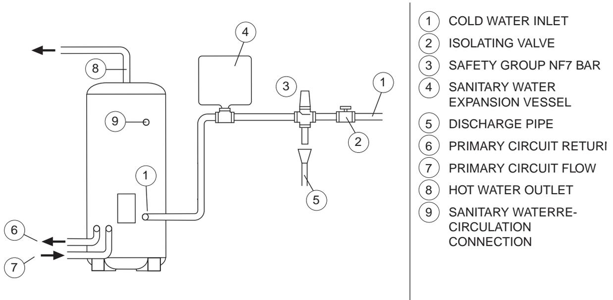
**Typical discharge pipe arrangement**
