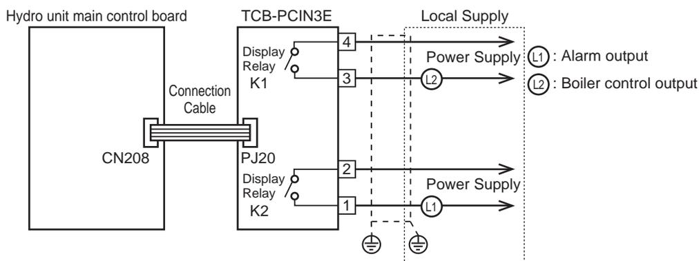
Operation output : Display relay is ON with outdoor unit compressor operation.
