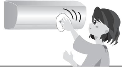
**Normal care :** Turn off power supply before checking or cleaning.
