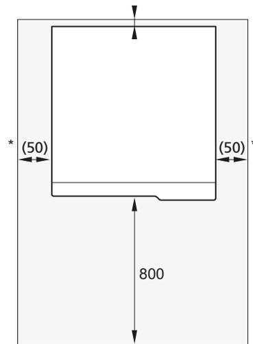
\* A normal installation needs 300 - 400 mm (any side) for connection equipment, i.e. level vessel, valves and electrical equipment.
