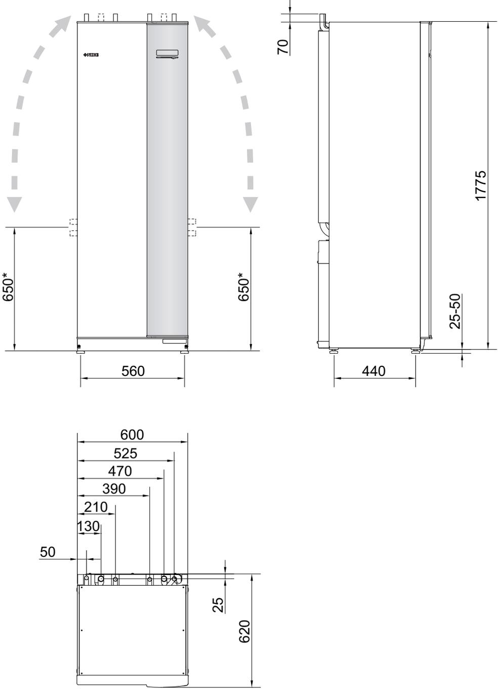
\* This dimension applies at 90° angle on the brine pipes (side connection). The dimension can vary approx. ±100 mm in height as the brine pipes partially consist of flexible pipes.
