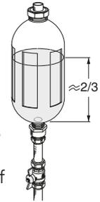
The pressure is raised by closing the valve on the incoming main line when the brine pump (GP2) is running and the level vessel (CM2) is open, so that liquid is drawn down from the vessel.
