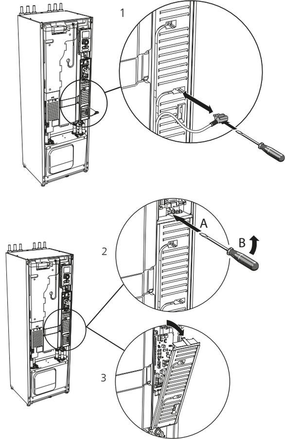
1. Disconnect the switches using a screwdriver.
