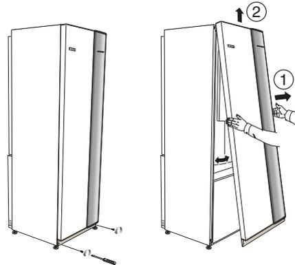
1. Remove the screws from the lower edge of the front cover.
