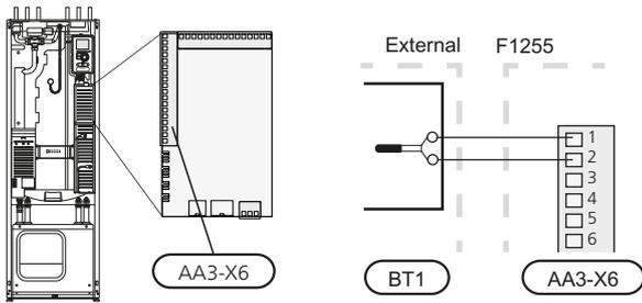
If the sensor is to be used to change the room temperature in °C and/or to change/stabilise the room temperature, the sensor must be activated in menu 1.9.4.
