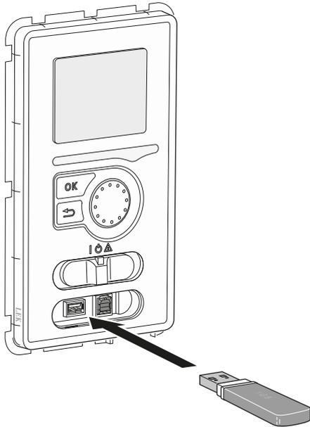
F1255 is equipped with a USB socket in the display unit. This USB socket can be used to connect a USB memory to update the software, save logged information and handle the settings in F1255.
