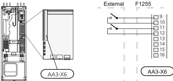
The example above uses the inputs AUX1 (X6:9-10) and AUX2 (X6:11-12) on the input circuit board (AA3).
