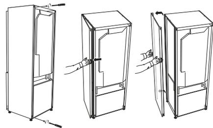
The side covers can be removed to facilitate the installation.
