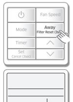
When maindicator is displayed, clean the filter and insert the filter back. After inserting the filter back, press the AND button for more than 3 seconds to reset the filter timer.
